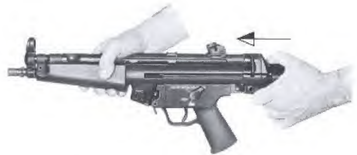
Fig. 35 Assembling the submachine gun
